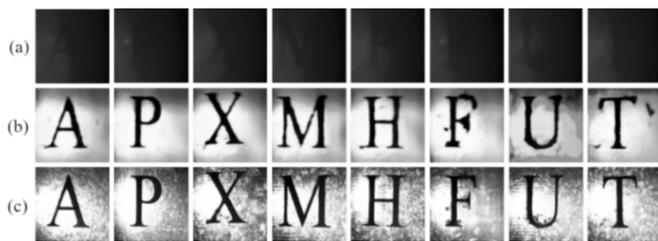
**Fig. 7.** Visual demonstrations of our Meta-DNET-UPI reconstruction on untrained letter targets. (a) The scattering image  $I_0(x, y)$ . (b) The images recovered by our Meta-DNET-UPI. (c) Ground truths.
