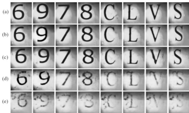
Fig. 9. Visual demonstrations of our Meta-DNET-UPI reconstruction on targets of different underwater imaging distances. (a) 8 cm. (b) 9 cm. (c) 10 cm. (d) 12 cm. (e) 13 cm.
