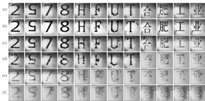
Fig. 10. Visual demonstrations of our Meta-DNET-UPI reconstruction on targets at different underwater turbidity levels. (a) 119.8NTU. (b) 133.3NTU. (c) 148.3NTU. (d) 162.1NTU. (e) 174.3NTU. (f) 187.1NTU.
